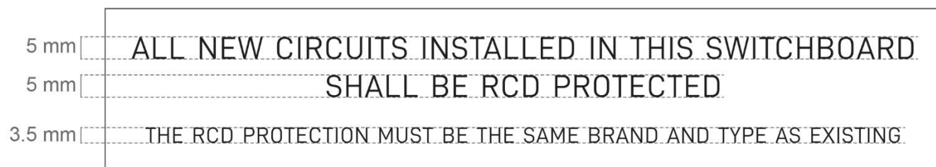
Figure 1. Label to display on all new Department of Education's school distribution switchboards (not to scale)
