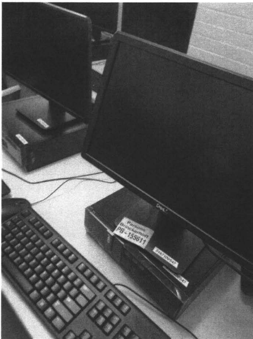
Sample PB-155611 Top of computers, south-western corner under ceiling penetrations and conduits. Dust found to contain Chrysotile and Amosite asbestos fibres.
